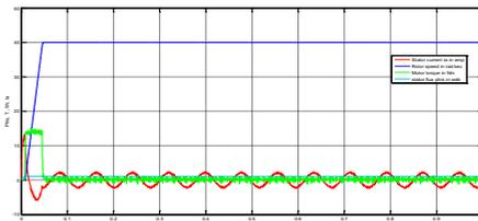
**Fig.14 Rotor Speed, Motor Torque, Stator Current and Stator Flux magnitude results of MRAS observer based SVM-DTC**
