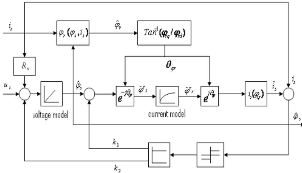
Fig.4 Sliding Mode Flux Observer.
