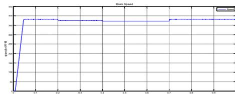
**Fig.11 Torque and Speed results of MRAS observer based SVM-DTC**
