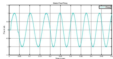
**Fig. 8 d-axis and q-axis stator fluxes of SVM-DTC**
