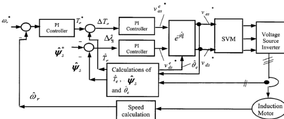
Fig.1 DTC-SVM based induction motor drive
